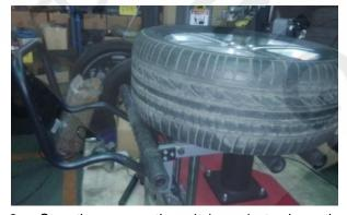
Step the pneumatic switch again to down the lift and tire.
