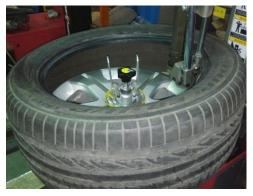
3. Lubricate the tire lip and rim then press the tire lip using the press disc to the below of the rim edge.
