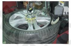
Return the press plate and demounting head. Finish the mounting.
