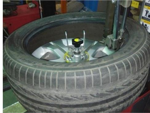
3. Lubricate the tire lip and rim then press the tire lip using the press disc to the below of the rim edge.
