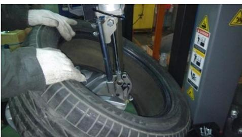
2. Rotate the main shaft clockwise to mount the downside of the tire.
