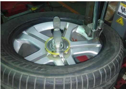
7. Lift the tire using the lower press disc.
