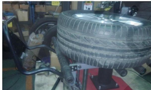
6. Step the pneumatic switch again to down the lift and tire.
