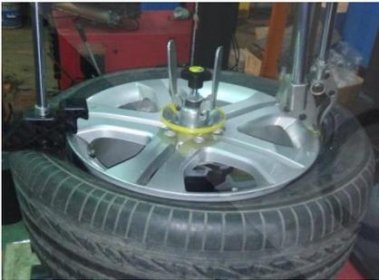
6. Rotate the main shaft clockwise to demount the upside of the tire.
