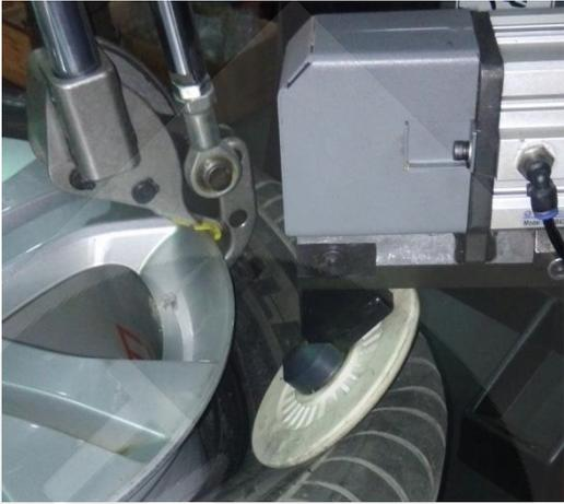
Pull the control valve downward to insert the hook into the tire.
