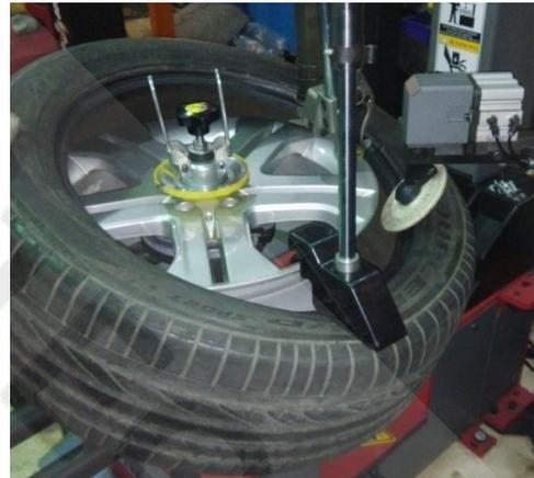
4. Rotate the main shaft to mount the upside of the tire.
