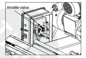
Fig 26 Valve mounting board
