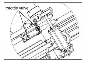
Fig27 direction switching cylinder
