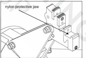
Fig 28 Mount the nylon protective
