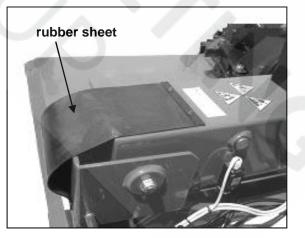
Fig22 Chuck protective rubber sheet
