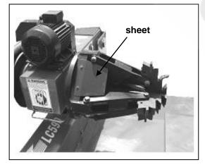
Fig21 Chuck protective sheet
