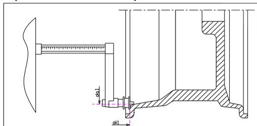
**Picture F16.8: Automatic acquisition of the internal plane distance and diameter in ALS2 Program Type**
