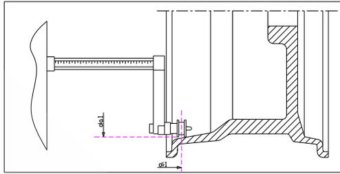
**Picture F16.9: Automatic acquisition of the external plane distance and diameter in ALS1 and ALS2 Program Type**
